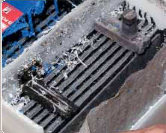
Plates are held in a micro-porous separating 'envelope'; glass fibre mat helps press the lead oxide firmly in the grid
