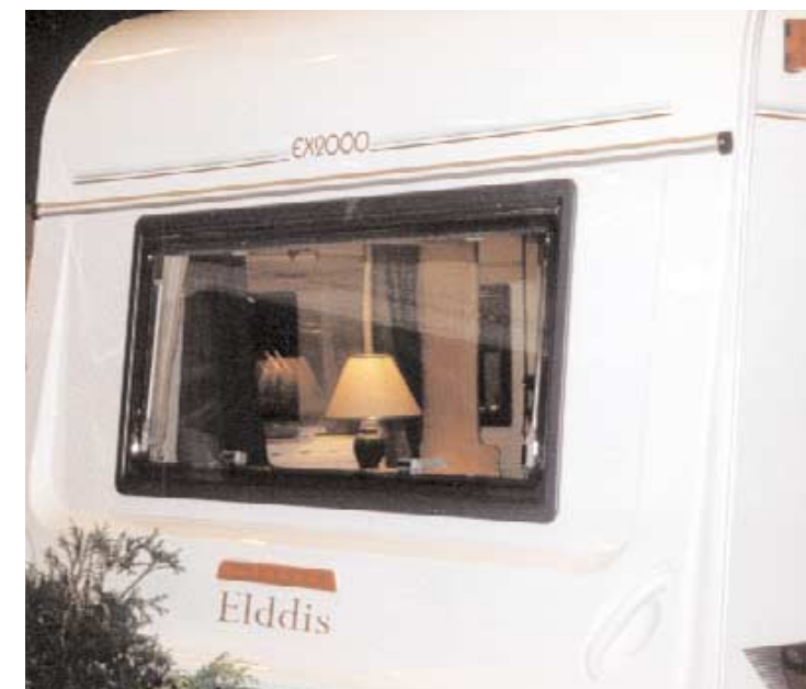
BELOW: Although framed acrylic window systems from Seitz are fitted to some caravans, they're more commonly seen on motorhomes
