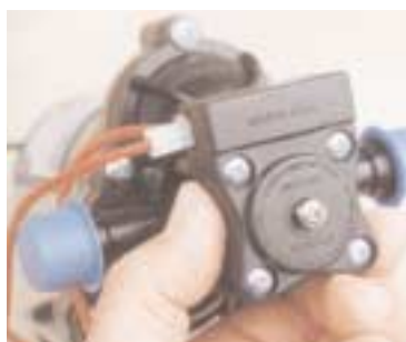
ABOVE: On the Shurflo TrailKing 7 diaphragm pump, pressure sensitivity is adjusted by the central screw
