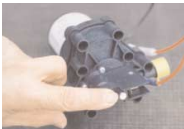
RIGHT: The pressure sensitivity adjustment screw on this Whale Evenflow pump is hidden behind protective silicon sealant
