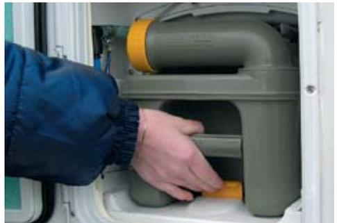
2. Remove cassette, ensuring the flap is in the closed position, and place on a trolley if required.
