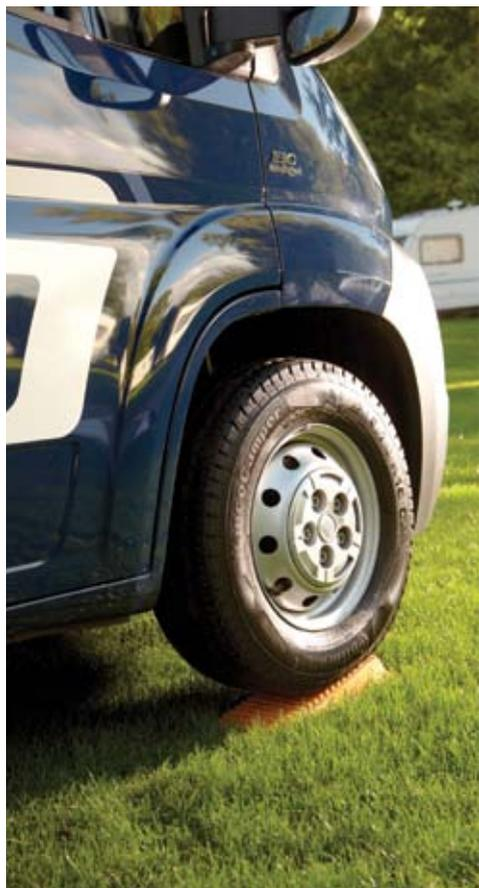
A glance at your pitch should tell you if you need side to side levelling. Reverse onto your pitch a foot or so further back than you want to end up, then place the levelling ramp in front of the wheel that needs to be raised. Place a spirit level parallel to the axle or the door. It helps to have two people at this point, one to drive the motorhome very slowly forward up the ramp, and the other to indicate when the spirit level bubble is in the middle. Chock the raised wheel for safety.
