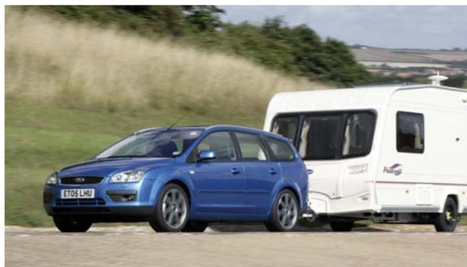
A laden caravan pushes down onto the car's towball. This is called the 'noseweight'. The optimum noseweight is generally 7% of the caravan's laden weight, so before buying a caravan, check this isn't in excess of your car manufacturer's stated limit.
