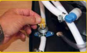
2. Some touring caravans and many larger motor caravans have a Trumatic Combi space/water heater. Combis have an automatic drain valve which triggers at 2°C-4°C but there's a manual control, too
