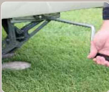
Corner-steady spindle threads only need a light smear of grease; large lumps attract grit
