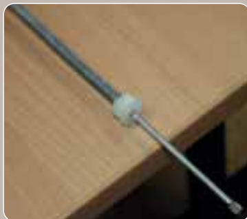
There's no need to withdraw a spring assembly like this but the illustration shows what's inside
