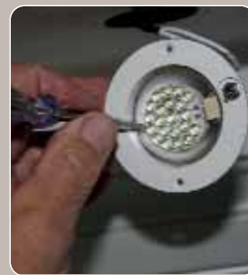
Great care is needed to avoid snapping the terminals; a screwdriver helps push this unit into place
