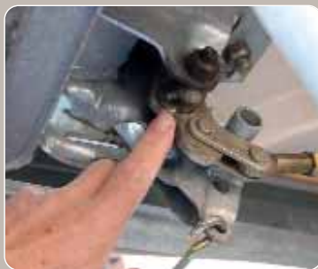
Grease nipples like this one on the underside of a coupling head assembly sometimes get missed
