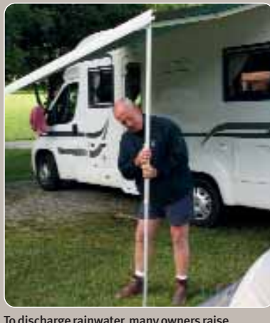
To discharge rainwater, many owners raise one pole higher than the other
