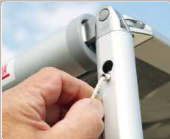
Each articulated, telescopic leg and side arm on a Fiamma Caravanstore stows inside the roller tube
