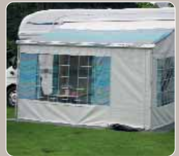
The cassette of this canopy awning on an Auto-Trail Cheyenne coachbuilt is mounted within a recessed channel
