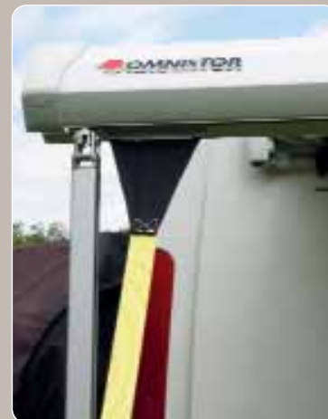
A groove under the fascia plate at the front of this Omnistor blind offers attachment for storm tapes
