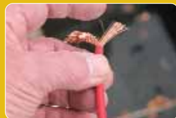
Counting copper strands can reveal cable rating
