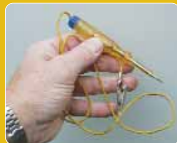
Cheap 12V testers have a translucent handle that contains the test lamp
