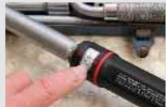
■ It is not unknown for wheels to become detached from caravans. That's why you are urged to have the wheel fixings checked with a calibrated torque wrench in accordance with the manufacturer's guidance.
