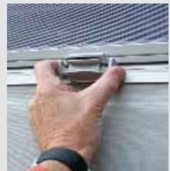
■ Against manufacturers' advice, many owners keep window roller blinds closed during storage periods. This can weaken the recoil spring. Check its operation because it may need re-tightening.
