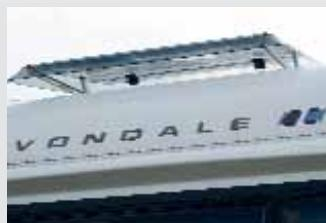
■ Rooflights usually need cleaning inside and out. Over time, dust gets blown under the frame and spiders often take up residence. Before towing, it's important to check the catches to ensure they engage with the frame.
