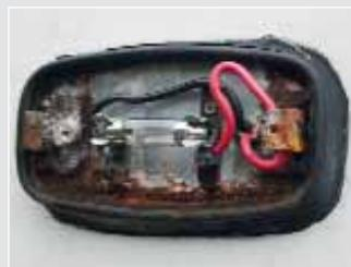
■ Driving rain can get into a caravan's road light clusters and damage the contacts. Marker lamps are similarly affected and the fittings on this motorhome were badly rusted inside.
