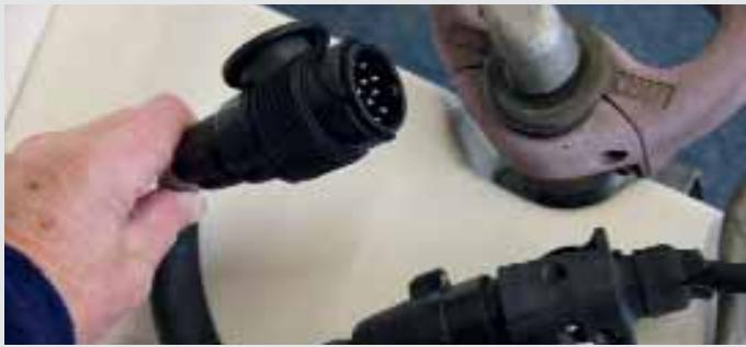
■ Irrespective of whether your caravan has seven-pin plugs, the more recent 13-pin plug or an adaptor cable, check road light operation well before departure. Car sockets often get dirty and damp inside and contacts may need cleaning.
