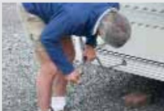
■ Confirm that corner steadies raise and lower with ease. Threads can seize up during long storage periods and the cure is to remove old grease, use a wire brush to remove grit and then apply a thin film of new grease.
