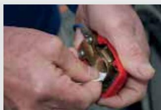
■ Leisure batteries are often transferred to a shed or garage where they can be left on a permanent trickle charge. Before returning a battery to a caravan, check the level of the electrolyte in each cell and clean the terminal connectors.
