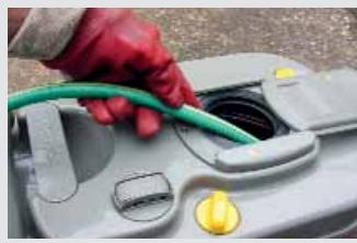
■ It's a good idea to hose out a cassette toilet but take care because a high pressure flow of water can damage its float mechanism. Then smear the rubber seal with olive oil or Thetford's seal fluid.
