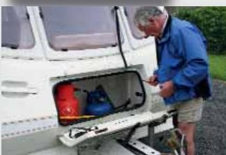
■ Prior to storage, many owners transfer gas cylinders to a well-ventilated, safe and secure place at their homes. When reinstating a cylinder, check the date on the flexible gas hose and consider booking a system leak test.
