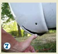
5 Side skirts and the moulded rear light panel on this Dethleffs model are made in ABS plastic 6 This new Kon Tiki Voque is clad in GRP sheet which can be repaired by skilful plastics specialists 7 If a replacement ABS panel is unavailable, damage like this can be repaired and it's not difficult 8 Replacing a damaged panel on an Airstream caravan would be a iob for skilled panel beaters
