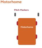
To avoid the spread of fire there must be at least 6 metres between facing walls of adjacent outfits, and 3 metres of space in any direction.
