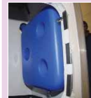
A small diesel fuel tank fitted in a caravan locker will run a heater that can operate safely while you're towing
