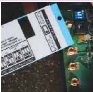
Sterling chargers often include setting switches so they can be used with gel and other sealed batteries
