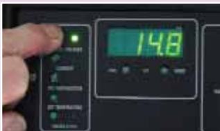
When a control panel indicates that your battery is receiving 14.8V, don't switch on any 12V accessories
