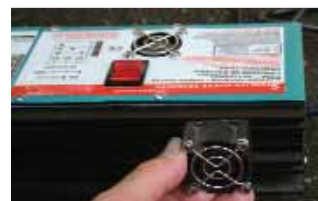
High-output chargers can get hot and are fitted with cooling fans. When operating, these might be noisy
