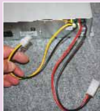
The BCA Leisure duo voltage charger has a battery connection producing 14.2V and an appliance supply of 13V
