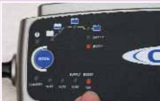
This particular CTEK stage charger includes a 16V output 'boost' to revive badly discharged lead/acid batteries
