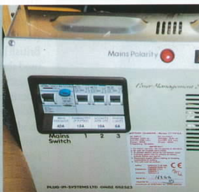
RIGHT: Consumer units fitted in caravans and motor caravans have a test button which you should push each time you hook-up, to confirm that the RCD's automatic disconnection facility is working correctly
