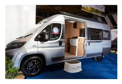
On the road price: £47,005 Extras fitted: None Number of berths: 2 Number of designated travelling seats: 2 Price as tested: £47,005 Base Model: Fiat Ducato Engine capacity: 2300cc Engine: 128bhp/130PS Fuel: diesel Gearbox: manual
