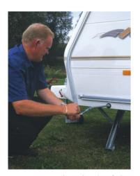
Lower the corner steadies to ensure they operate easily, are well maintained and not bent through misuse. Ask to take the caravan for a trial run and note its behaviour on the road, in particular that the overrun brakes work smoothly. An overrun brake is one that
