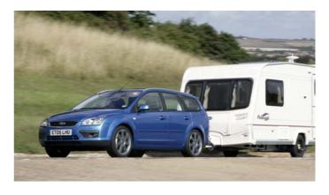
A laden caravan pushes down onto the car's towball. This is called the 'noseweight'. The optimum noseweight is generally **7**% of the caravan's laden weight, so before buying a caravan, check this isn't in excess of your car manufacturer's stated limit.
