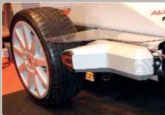
The Al-Ko Mammut is neatly enclosed and there's no loss of clearance on the integrated chassis model
