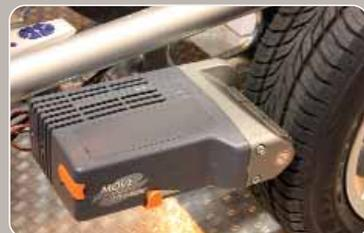
The specification on this Reich Move Control Compact states it moves single-axle caravans weighing up to 2000kg
