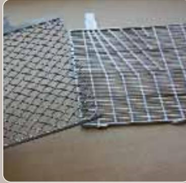
Plates use a grid of lead, and on a leisure battery this is stiffened with antimony; calcium is used in car batteries
