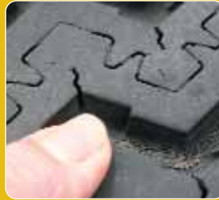
Another indication of tyre depreciation is cracking between the treads
