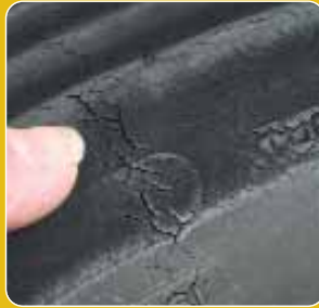
Pay particular attention to the sidewalls of tyres; cracks like this are a sign of pending failure
