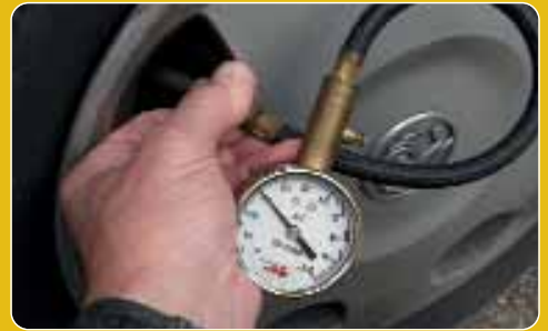
Robust dial-type gauges are often recommended by specialists
