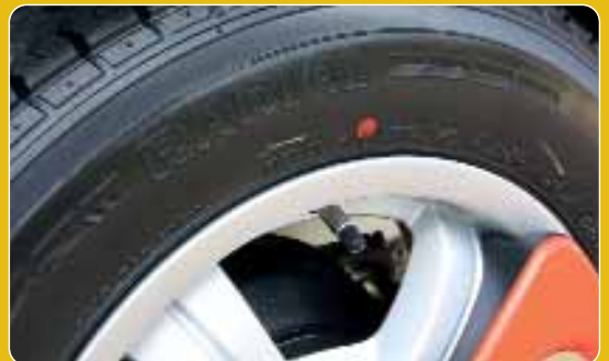
The last two digits on this caravan tyre's 185/70R14 size designation confirms it's for 14in rims
