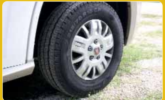
This motor caravan has 15in diameter rims and its tyres bear the 'Camper' (CP) designation
