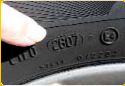
The 2607 mark on this motor caravan tyre indicates that it was manufactured in the 26th week of 2007
