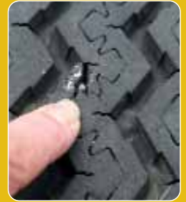
It's surprising how often a tyre inspection reveals sharp objects trapped in the treads
