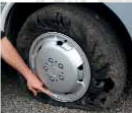
This tyre is ruined but its Tyron band ensured that the tread remained in constant contact with the road
