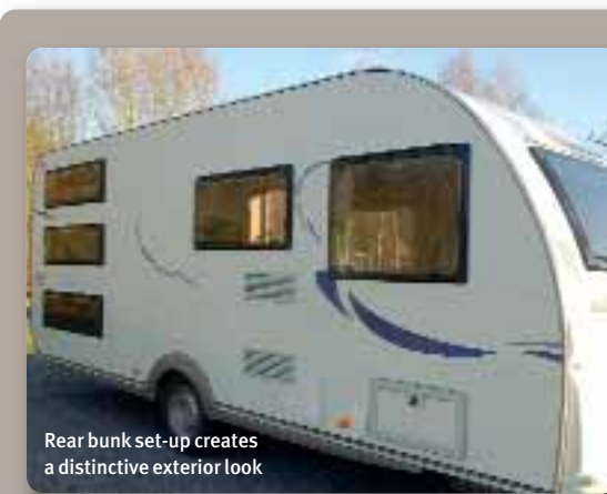
Sides are polyester while front and rear are ABS plastic
