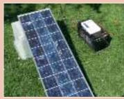
This is one of the more common, rigid types of solar panel, which has an aluminium frame and a toughened-glass protective covering.
