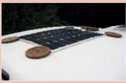
Weights are used to hold the panel down while the adhesive cures. Further sealant is later added around the perimeter to seal the junction between the roof and the panel. The cable entry point is also sealed.
