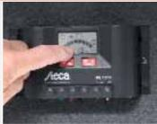
To prevent battery over-charging, a regulator is usually needed. Some are inexpensive but many owners want one with a screen that indicates charge levels, an Ah summary and so on.
