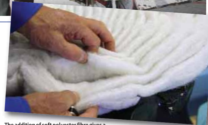
The addition of soft polyester fibre gives a rounded shape to sharp-edged foam
