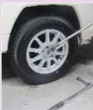
Wheel fixings are checked with a calibrated torque wrench, then re-checked by another technician using a second wrench
