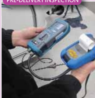
A probe is inserted into gas flues to gather information about the presence of CO and CO 2 from appliances
