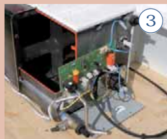
3. Electronic controls are commonplace and operation relies on a good 12V supply
