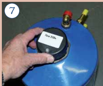
7. Some combined Eberspächer systems include a copper cylinder with a 230V immersion heater
