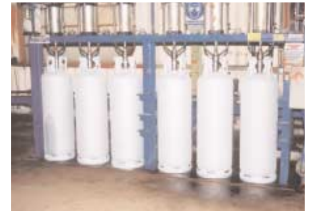
In the kerosene leak test, the cylinder on the far left is weeping
